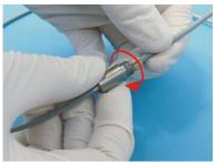
2. Unscrew the chuck from the fixing sleeve and pull the chuck with the fixing sleeve from the transmission fibre optic conductor.
