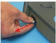
To charge the battery, connect the wireless foot switch to the power supply by means of the charger adaptor included in the delivery.
