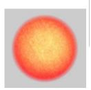
6. Direct the distal end of the transmission fibre optic conductor (distance: approx. 20 mm) vertically to a bright, flat surface and observe the light spot of the pilot laser beam (radiation characteristics).
