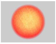
13. Switch on the laser device. Direct the distal end of the bare fibre tip (distance: approx. 20 mm) vertically to a bright, flat surface and observe the light spot of the pilot laser beam (radiation characteristics). If necessary, check the screw connections of the clamping on the handpiece.
