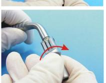
Remove the tool with sapphire tip from the pack, avoiding contact with the sapphire tip.
