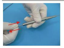
**12.**Verify the firm seating of the transmission fibre optic conductor.
