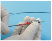
Guide the transmission optic fibre conductor through the opening in the fixing sleeve.
