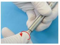
Unscrew the fixing sleeve from the handpiece completely and pull the transmission fibre optic conductor with the chuck and fixing sleeve slowly from the handpiece.
