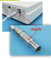
Observe the position of the plug when you connect the charger adaptor:
