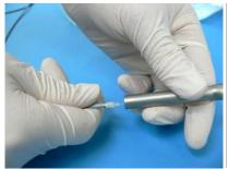
**8.** Guide the transmission fibre optic conductor with the mounted bare fibre tip into the handpiece.
