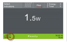
If the battery charging is inadequate, a symbol will appear at the bottom of the screen on the left. From this time, the foot switch will remain in operation for approx. 5 hours. Charge the battery after completing the running therapy.
