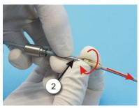
3. Guide the optic fibre conductor through the opening in the chuck and screw the chuck onto the fixing sleeve (2) of the optic fibre conductor.
