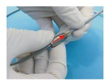
Mount the fixing sleeve, applying slight pressure to the chuck.
