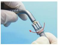
**3.** Unscrew the sapphire tip from the handpiece using the tool.
