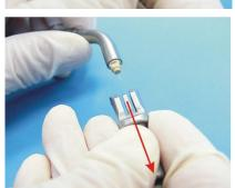
**8.** Screw the sapphire tip into the handpiece in a clockwise direction.
