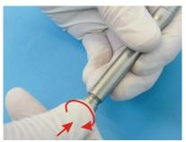
Screw the fixing sleeve at the proximal end of the handpiece so that the fibre optic conductor will still have freedom of movement.
