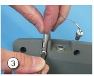
Screw both ends of the bracket tightly to the foot switch, fastening the sealing cap of the bush.
